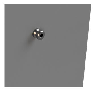
Take the FX-10030-BLU fixing and screw into the aluminium skin using a 6mm Allen key until this sits flush with the face of the door.
