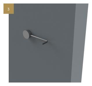
You can use the small location hole to insert a small Allen key to allow you to tighten the bolt up against the Brass Ferrule.
